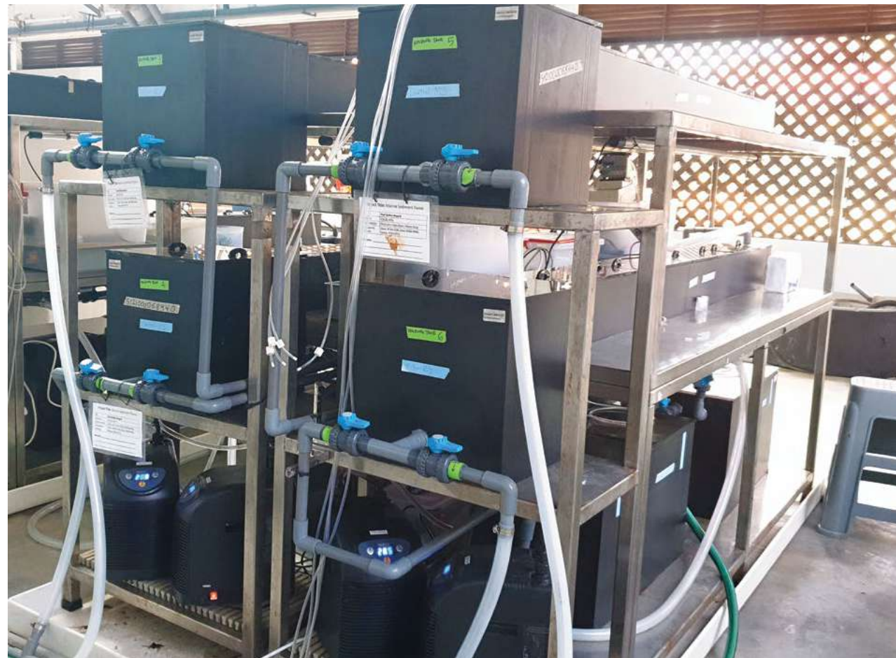
Figure 1: Flume mesocosms with water quality sensors. Six 2 m-long rectangular flumes were seeded with sediments from areas not impacted by aquaculture; subsequent biofilms were developed over three weeks before adding the three target organisms.
